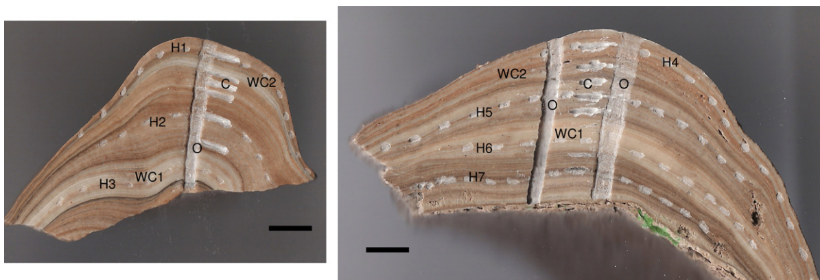
Fig. 2. Stalagmites Asfa-3 (left) and Merc-1 (right). δ 18 O profiles are vertical suites of samples labelled ‘O’ (duplicate analyses on Merc-1). Samples for Hendy tests are horizontal drill samples along laminae (labelled ‘H1–7’; three on Asfa-3, four on Merc-1). Five 14 C analyses (label ‘C’) are also visible on each sample (the sixth analysis is on the stalagmite top). 1 cm scale bars shown.
